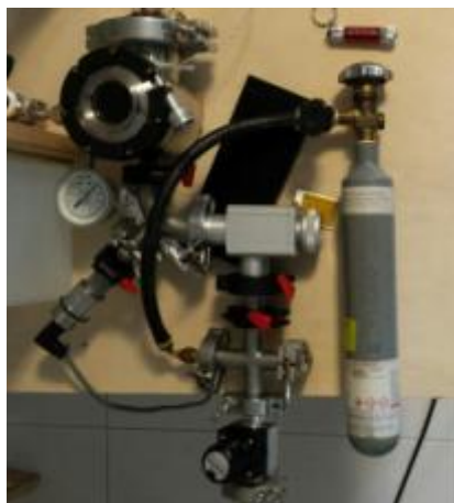
Reactor 1 with the material inside; configuration to fill D2 gas; sample with Pd deposit (II test)
